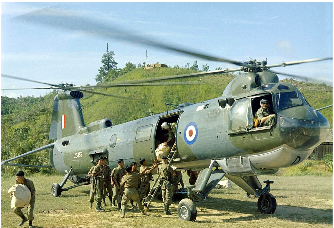
Based on the Type 173, the Bristol Type 192 entered service as the Belvedere HC Mk1 in 1961
